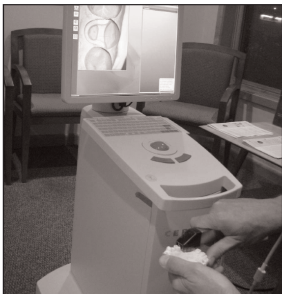
Figure 1. Dr. Phelan scanning a cast into the CAD system, which simulates scanning a tooth for which a cap is to be made and fitted.
