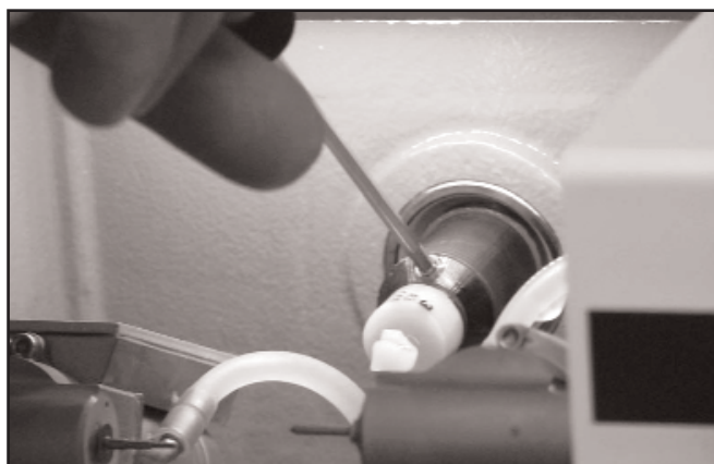
Figure 2. Dr. Phelan removing the finished implant from the milling machine spindle.
