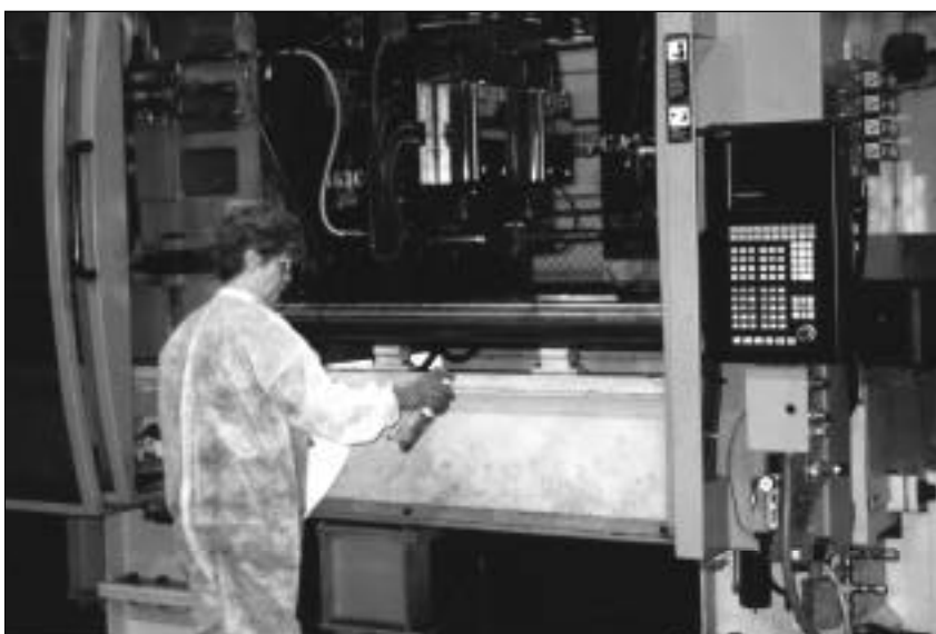
Figure 5. Cell team member conducting a TPM on a 700-ton injection molding machine.
