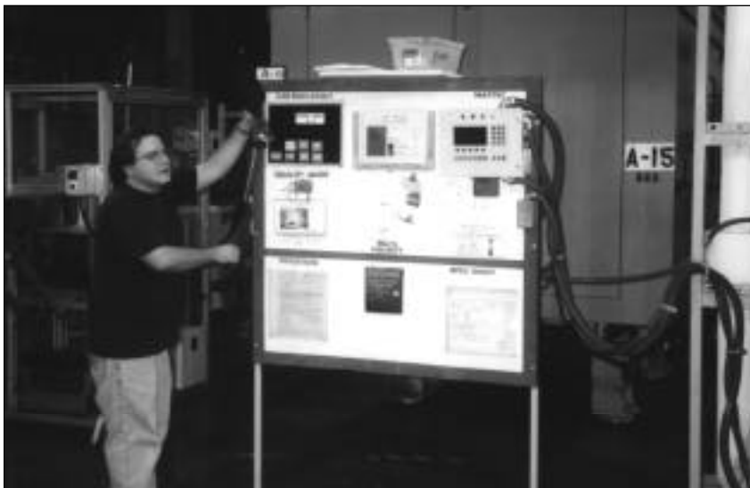
Figure 4. Every workstation has a Kanban board featuring visual tools signaling recent performance; an associate is changing flags used to indicate scrap status.
