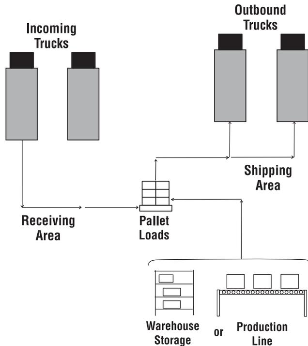
**Figure 5.** Incoming materials are blended with items coming from onsite storage to complete outbound loads. If the warehouse is co-located with a manufacturing facility, items coming off the production line may be sent directly to pallet make-up to be blended with items coming off arriving trucks. In some instances, some incoming materials may also be routed to storage instead of all being crossdocked immediately.
