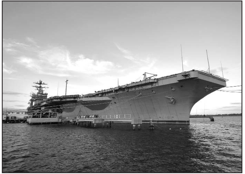
Figure 4. The Nimitz-class USS Harry S. Truman (CVN-75) at the Lambert's Point Deperming Station in Norfolk, VA. While at the station, the ship was wrapped with electrical cables which are charged with a current that removes the magnetic field from the ship. Demagnetizing ships counters magnetic mines and stops interference with communication and navigation equipment.
