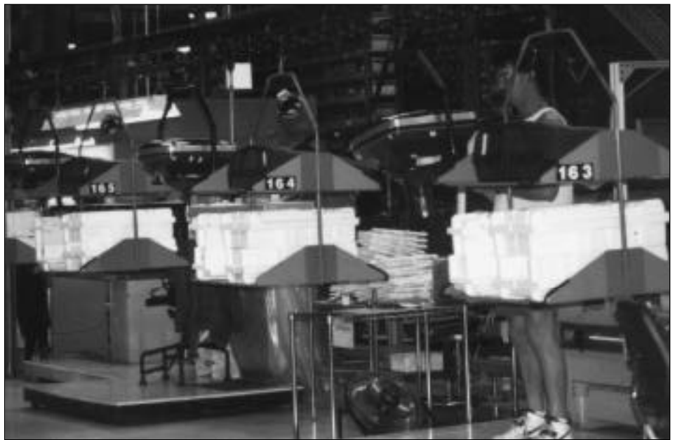
Figure 4. The JIT delivery system for packaging material to final color TV packing stations.
