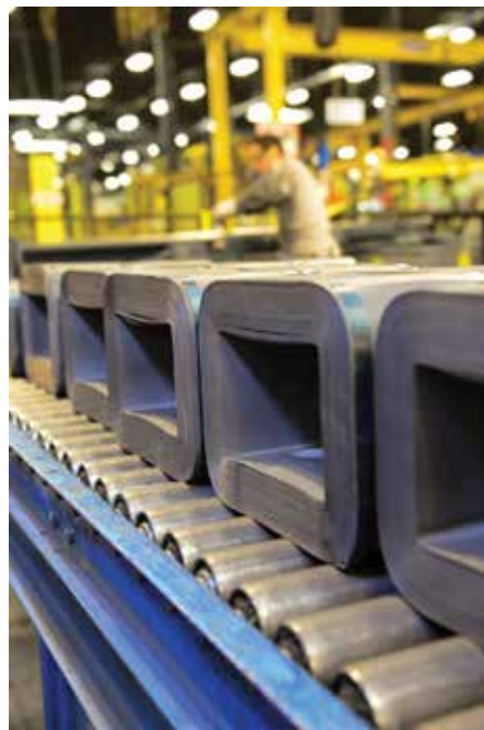
Cores for distribution transformers.
