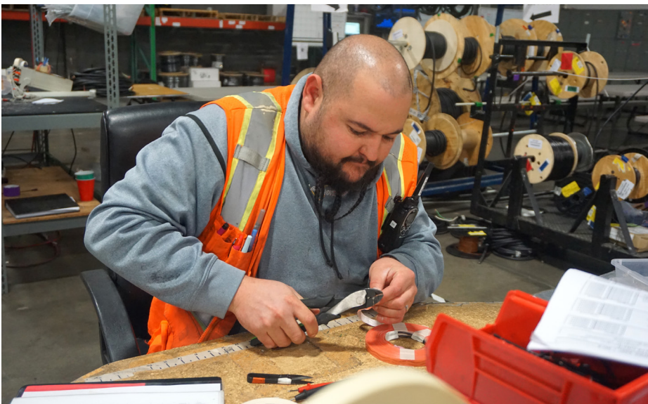
Jaime Flores, floor production supervisor at Powerblanket, crimps the ends of a heater.
