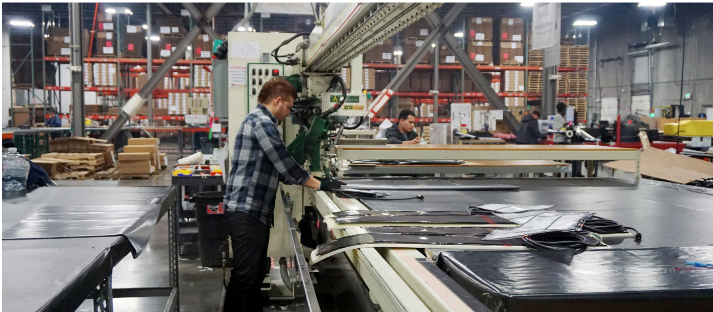
Moises Castillo, a new full-time hire at Powerblanket, heat welds the outer vinyl covering of our product.
