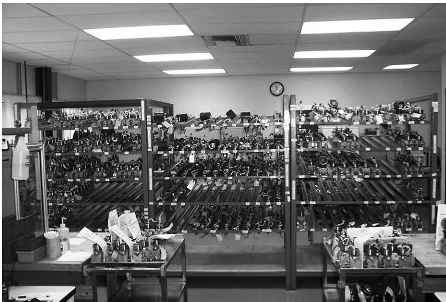
Figure 2. Invensys employees learned how to reduce order turnaround time and keep lower inventory on hand by setting up a supermarket to stock the 36 items accounting for 60 percent of a product line's sales. Products are customized and shipped within 24 hours of order receipt, offering a competitive advantage.
