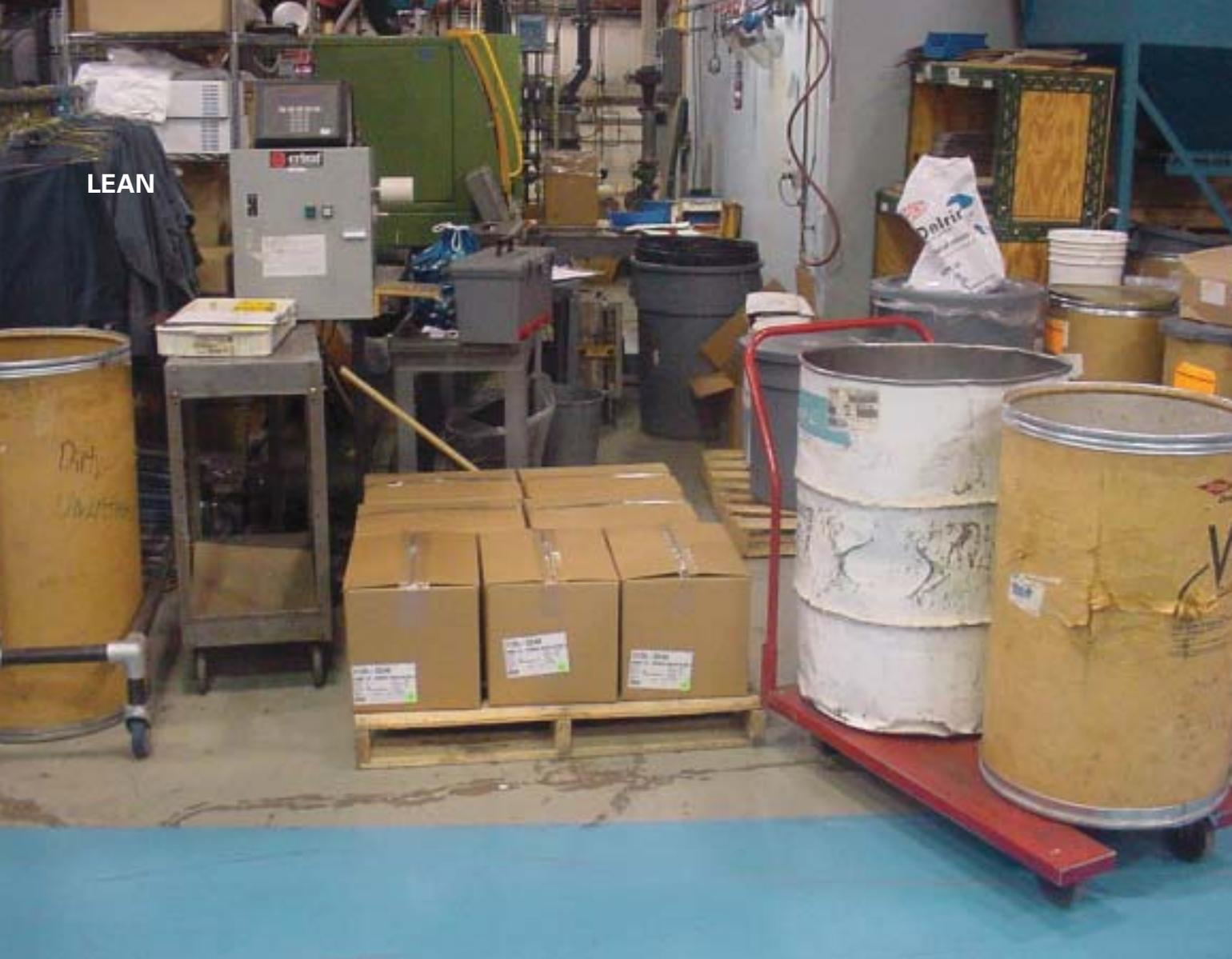
**HIDDEN FACTORY.** Here is a workplace where status of operation is not apparent and where wastes (transportation, inventory, motion, waiting, overproduction, overprocessing and defects) are prevalent.
